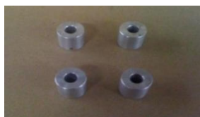
(4) Spacer Stanchions - used for different Mold Plate thicknesses. Material may be plastic.
