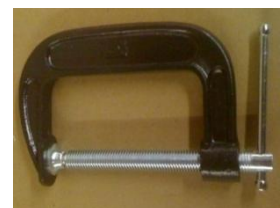
(2) Clamps. Used to secure machine to work table. Call factory for details.
